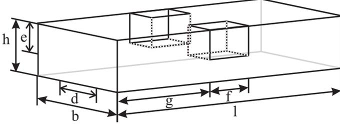
Figure 2: Setup - air filled waveguide with PEC implants. The dashed lines mark the edges where a correction factor is performed.
