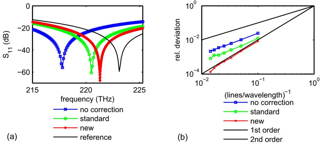
Figure 3: (a) Reflection coefficient  $S_{11}$  (10 lines/wavelength). (b) Relative deviation to the reference result (resonance frequency).
