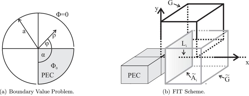
Figure 1: Setup for the analysis of edge singularities (a) and example FIT grid with used nomenclatur (b). The grid flux  $\widehat{d}_i$  is defined on the dual Grid  $\widetilde{G}$ , the grid voltage  $\widehat{e}_i$  corresponds to the primary grid  $G$ .
